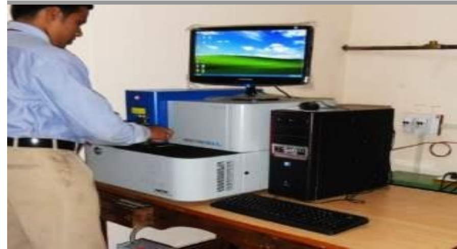
Spectrometer – 31 Elements including Nitrogen Facility
