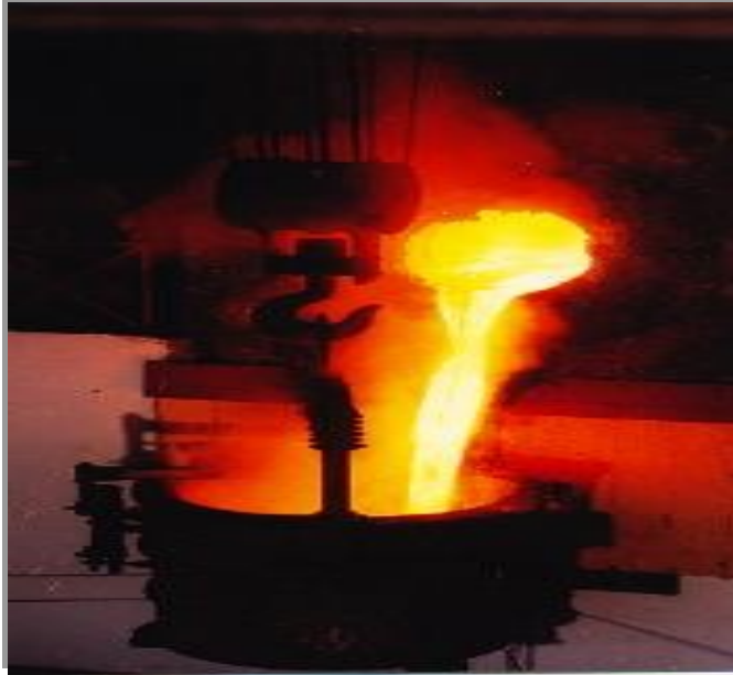
Induction Furnace - 12 MT
